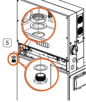
Gently plug in each battery module from the bottom up. Fasten the modules on both sides using M4x8 screws (Torque: 1.2 N·m).
