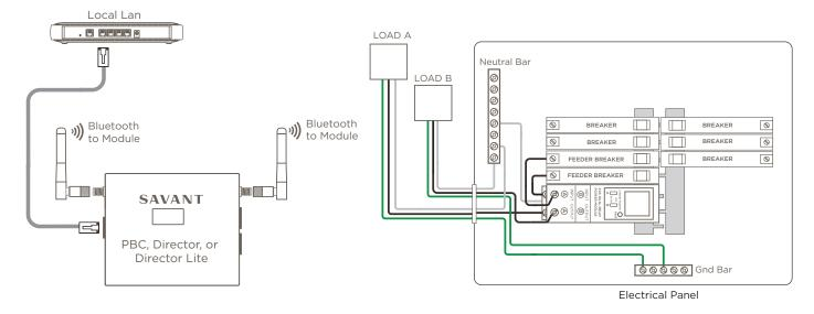
HELPFUL! The diagram shows an electrical panel that doesn't contain a plug-on neutral bus bar. However, both plug-on neutral and non plug-on neutral panels are supported
