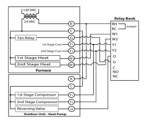
This system uses an indoor air handler with condenser for supplying heat and an evaporator for supplying cool. The system has a reversing valve to select whether heated or cooled air is produced. The system has two stage heating as well as two stage cooling.
