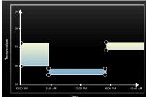
The schedule above is a fall schedule where the temperature from 12:00AM to 6:00AM is set to not go below 60°F and not go above 72°F. From 6:00 AM to 5:00 PM the temperature is kept between 55°F and 58°F. At 5:00 PM the temperature is set to stay between 68°F and 72°F
