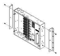
(2) Mounting Brackets (SMB-8000-00)(4) Mounting Bracket Screws 10-32 x ⅔ inch FH
