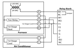
Two Stage Furnace with Air Conditioner
