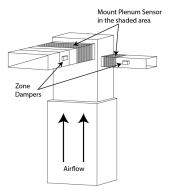
1. In the shaded area shown above, drill a hole into the ductwork.
