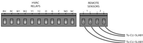
6. For information on configuring the sensors to communicate with the CLI-8000, refer to the CLI-SLAB1 - Configuration and Calibration section.
